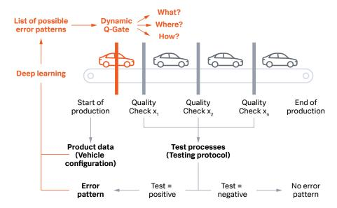
BMW manufacturing engineers ensure high production quality using insights from Splunk, which provides a holistic view of vehicle data during production. Using DSDL, the BMW Innovation Lab team identified benchmarks for different vehicle types and configurations using Uniform Manifold Approximation and Projection (UMAP), helping BMW generate baselines for expected behaviors
