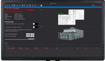
winhag alarm management system integrates with sub-systems to give excellent operability, intuitive control, and sequence automation. The system enables users to visualise and evaluate emergency situations for evaluation in 3D. WINMAG can control access and escape routes, while providing information on the status of equipment like elevators during evacuation.
